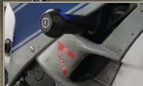
Puig frame-sliders come in handy whenever the pilot has to hit the eject button.
